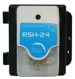
The Remote Strobe & Horn combines two alarm features, a visual and an audible into one compact, low profile device. It is powered by 24 VDC / VAC; connect 15 - 26 VAC /VDC at 500 mA to power this device. The current draw is approximately 350 to 450 mA.
